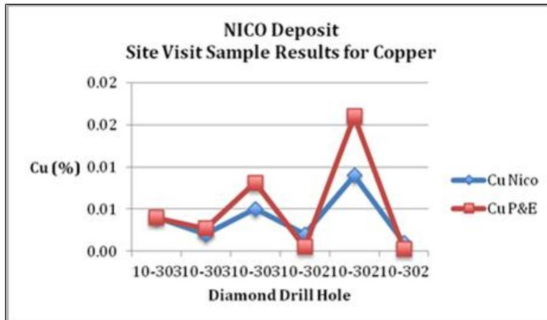
The check samples were collected by quarter-cutting the remaining half core in the core box. They were given a unique sample number, placed in a bag and, once all samples were collected, were placed into a larger bag and taken by Mr. Puritch to the offices of P&E in Brampton, Ontario. From there, the samples were sent by courier to AGAT Laboratories (AGAT) in Mississauga for analysis.
